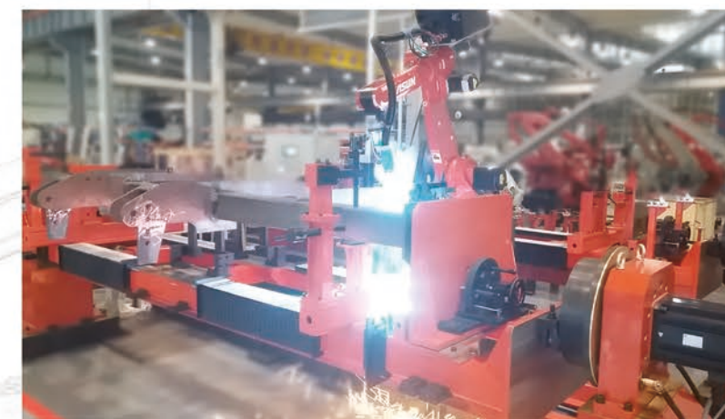
Welding of agricultural machinery base frame, main shaft and other components has been completed by robot
