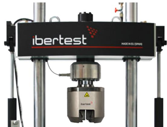
Example: Load cell  $\pm 250$  kN
