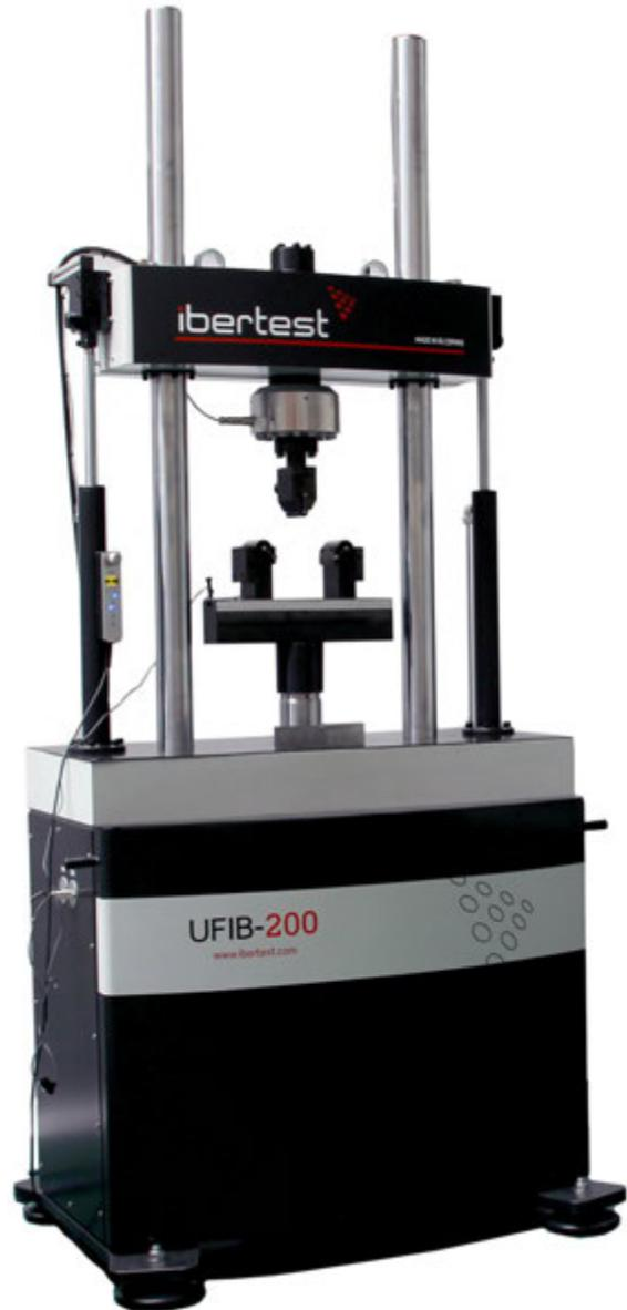
The mechanical design of testing frame is made with finite elements analysis using the design ANSYS software to determine, in addition to the analysis that guarantee the specified rigidity, those important parameters for the correct operation of the machine without resonance under dynamic conditions.
