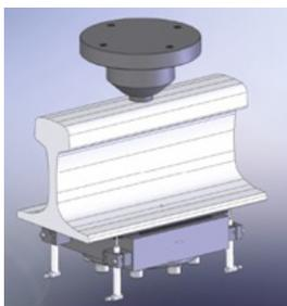
*Rigidity test over elastic plates for a high speed rail*
