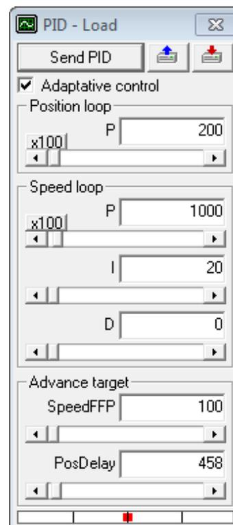
The PID parameters depend on the type of control and on the tested specimen's mechanical characteristics and on the working frequency. These parameters may be modified during the test and should not be changed abruptly. The modifications are carried out through a window enabled with that purpose on the main panel shown when the dynamic data display is enabled.
