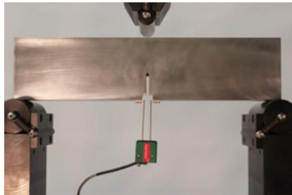
Fatigue three point bending test with fracture mechanics extensometer
