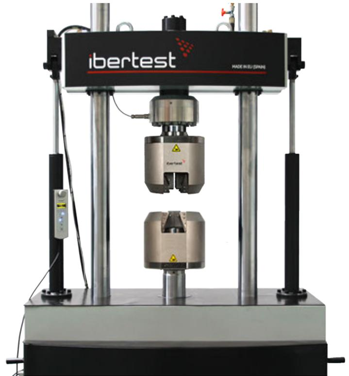
*Gripping heads, wedge type and hydraulic closure*
