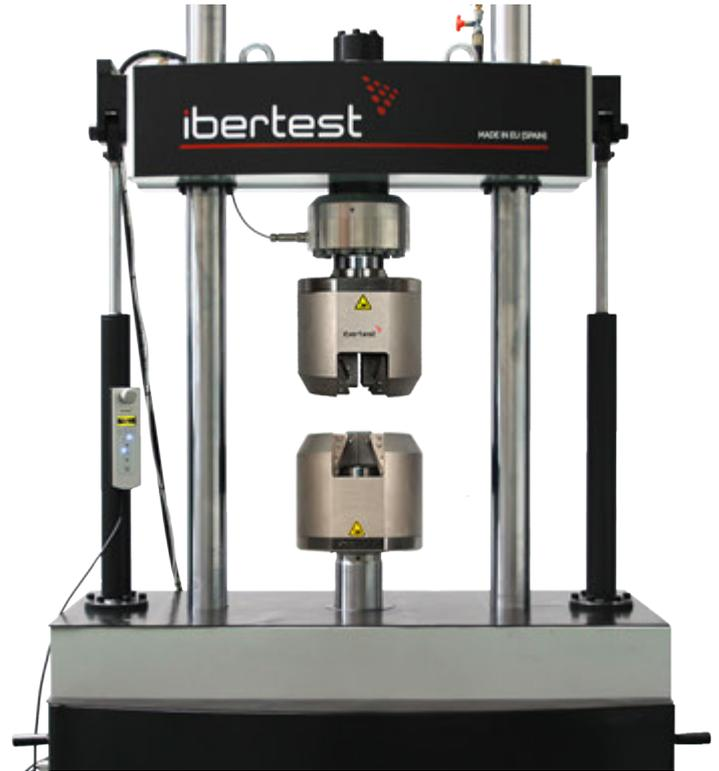
*Gripping heads, wedge type and hydraulic closure*
